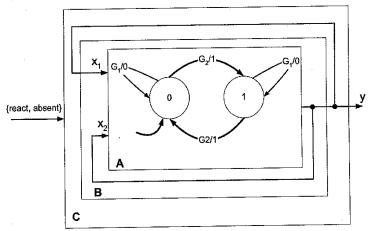
Let the set  $D = \{0, 1, absent\}$  denote an alphabet. For every pair  $(x_1(n), x_2(n)) \in D^2$ ,  $x_1(n)$  and  $x_2(n)$  denote the top and bottom input symbols in the figure, respectively. The  $n^{th}$  output symbol  $y(n) \in D$ .
