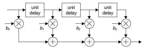
Suppose that this system has frequency response  $H(\omega)$ . Define a new system with the identical structure as above, except that each unit delay is replaced by a double delay (two cascaded unit delays). Find the frequency response of that system in terms of  $H(\omega)$ .
